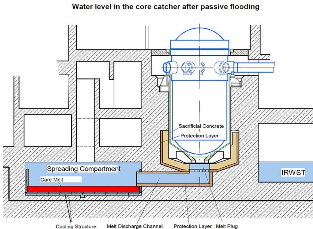
**Figure 4: Generation III SA management design for EPR, core melt spreading and cooling for ex-vessel melt retention (Wikipedia, 2013, Areva, 2009). However, analytical and experimental programmes that could confirm that concepts like the above core catcher actually work are still ongoing, and face potentially unresolvable methodological problems.**
